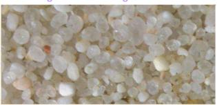
The outdoor extraction of the mine of wind-eroded dunes in Sanchonuño and an area surrounded by a pine grove (Segovia). It is washed under natural water with no chemical additives for his later classification with moisture contact, it is dried in a biomass oven and is dry calibrated. Silage process of the dried sand. It is a chemical additive-free product so we could say that it is an environmental silica sand. Furthermore, the product remains unchanged; it is only classified by dimensions.
